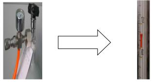
4. When the screen displays the calibration level, please inject the standard gas into the tester. The detector will automatically analyze the gas and process the calibration. After calibration, press to save. If need to make other gases' calibration, please repeat the above process.
