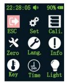
2. press into calibration, input the password 0000, Choose the gas type. Please note, make the calibration one by one.
