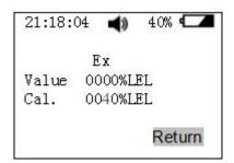
Note: The calibration point for Ex is 40% LEL by default. CO is 500ppm, H2S is 50ppm. Make the O2 calibration in the clear air.
